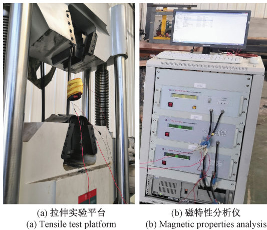
图 8 不同应力下 Q235 磁化曲线测试实验图 Fig. 8 Experimental diagram of Q235 magnetization curve under different stresses
